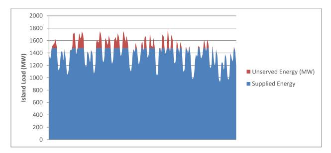
Figure 10: Change in Shortfall with Addition of Bay d'Espoir Unit 8
