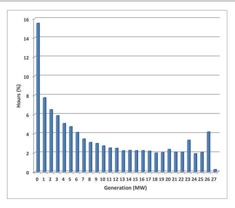
Figure 5: Fermeuse Generation from April to November (2010–2018)
